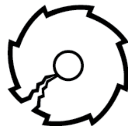
Inspect jammed blade for damage
